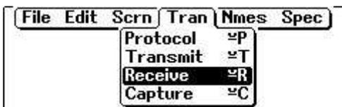
To start the receive operation press Menu again. Select Tran and arrow down to Receive and press Enter.
