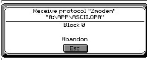
You should then see the following screen indicating that the receiving protocol is "Zmodem" and that the file ASCII.OPA is going into the APP folder on the A: drive of the Psion
