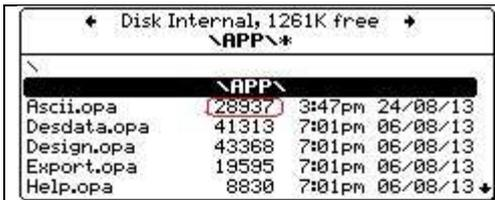
Once the transfer is done, it's a good idea to make sure that the file has gone through correctly. Easiest way is to check the size of the file on both the PC and Psion.
