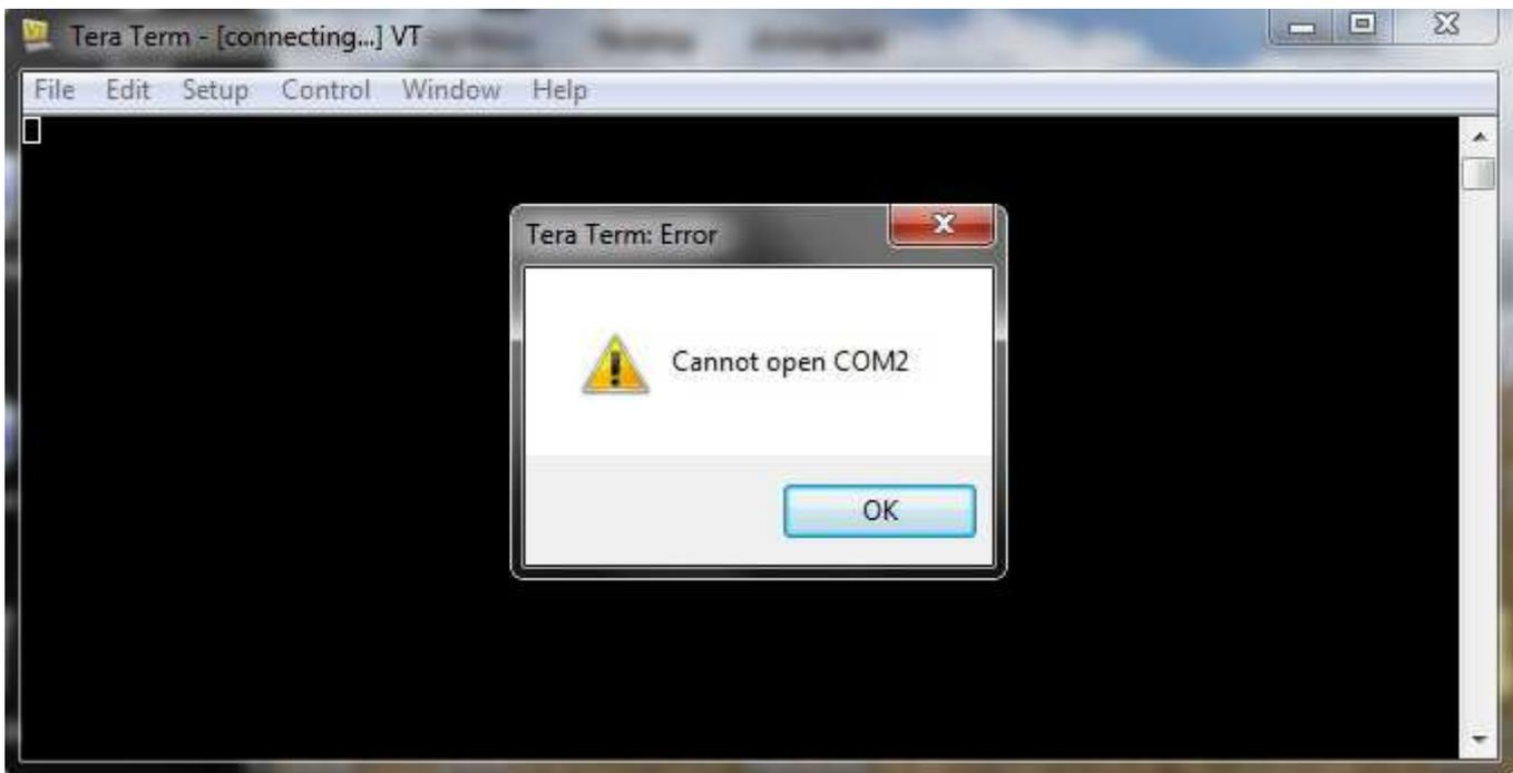
Its looking for a previous setting. You can either go to Device manager and see where the USB is installed or select **File – New Connection**
